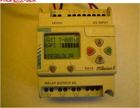
It is easy to mount PLC. You only mount cables from sensors and parts
